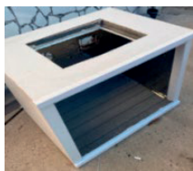
Figure 1. Chamber with internal dimensions of 0.7 x 0.5 x 0.5 m with a volume of 0.175 m 3
