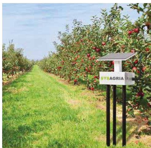
Figure 8. View of the multi sensors device with autonomous energy and wireless communication including soil pH measurement
