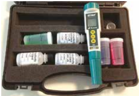
Figure 2. EC510 conductivity testing kit including: EC500 meter, 3 calibration standards, 3 pH buffer pouches plus rinse solution
