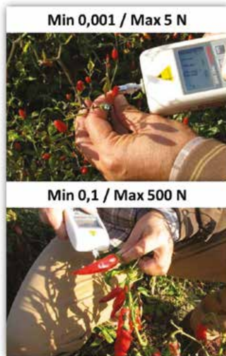
Figure 1. Measuring of FDF using push-pull digital gauge
